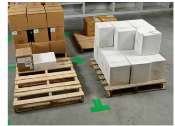
3. Colour-code material storage areas.
