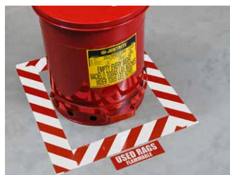
8. Colour-code hazardous areas or equipment.
