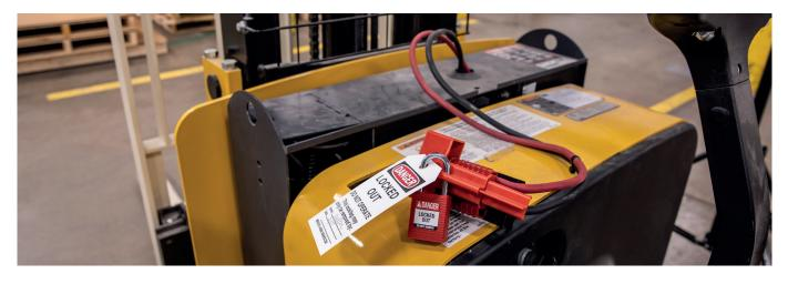
Easy to use and applicable on a wide range of industrial vehicles, the BatteryBlock Power Connector Lockout is a great addition to your maintenance safety tool kit.
