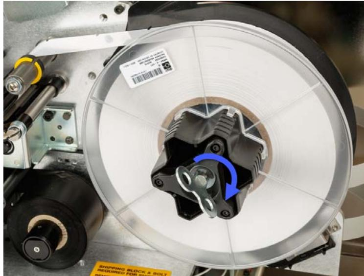
*Figure 4-3. Tighten Label Spool*
