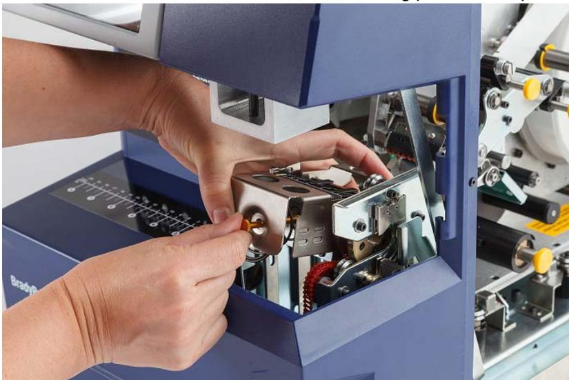
The front door was removed for better visualization. It is not necessary to remove door when replacing block assembly.
