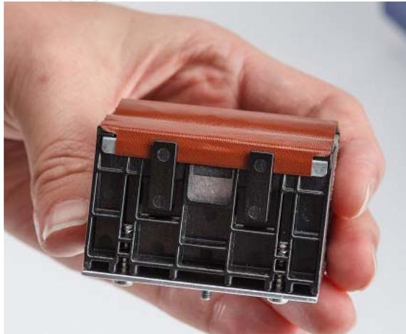
10. Insert the flagging block assembly so the black nubs and threaded stud line up with the holes on the mating surface. Hold the flagging block in place against the mounting surface.
