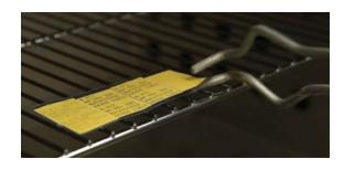
After 30 days in the elevated temperature, the samples are evaluated to see if the temperature had any negative effects on the print or the material. The samples are examined for any signs of fading, discoloration, shrinkage, adhesion loss, ooze, material embrittlement, or topcoat cracking.
