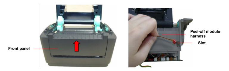
3. Plug in the peel-off module harness connector to the 5-pin red socket on the main board.
