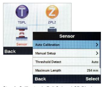
Step 2: Calibrate via Full Colour LCD Display
