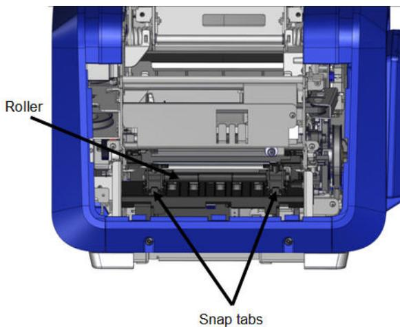
5. When free of the catches, lift the roller out.
