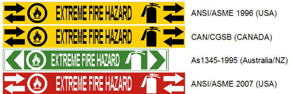
**Figure 13 • Color norms for Standard Pipe Markers**
