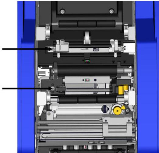
3. Using a pre-moistened foam swab, gently insert the swab under the media guides and wipe the surface of the sensors. Do not allow the alcohol to drip from the swab.
