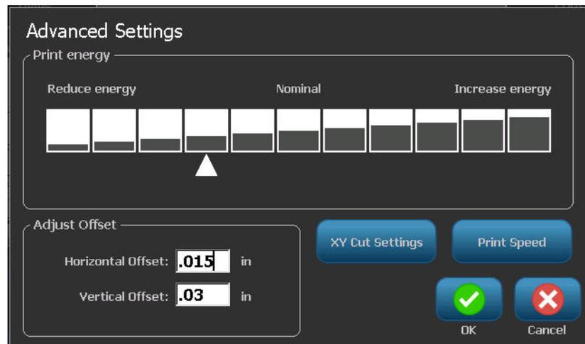
**Note:** By default, the print energy is at the nominal setting for the best overall performance. Because the nominal setting is programmed into the touch cell, the selected print energy setting stays in effect for all subsequent print jobs with the currently installed media. When new media is installed, the print energy level is reset to the default setting. The print energy level is also reset by rebooting the system.
