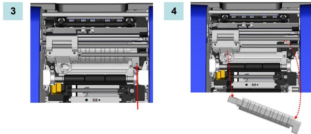
6. Remove the cut pad screws.
