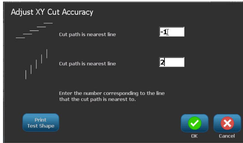
9. On the Adjust XY Cut Accuracy screen, touch Print Test Shape
