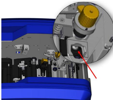
5. Using a cotton swab moistened with the Isopropyl alcohol, clean off any dust from the area where the blade sticks out.
