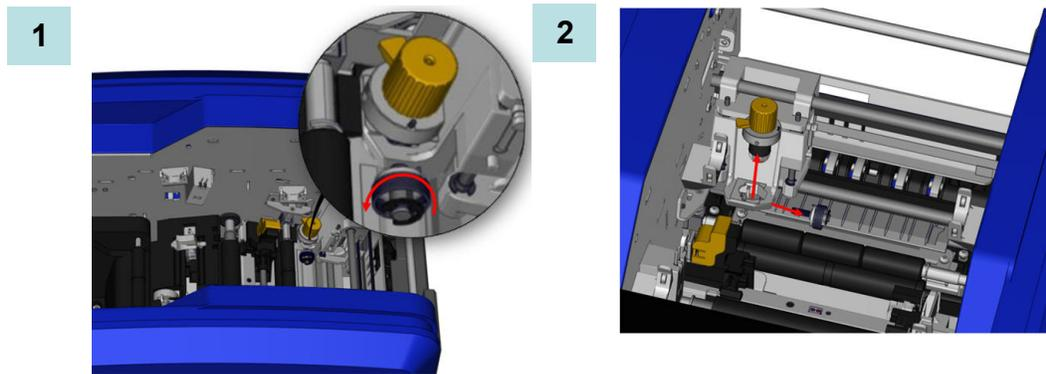
3. Using a magnetic screw driver (so screws do not drop into the printer) remove the upper guide screw.
