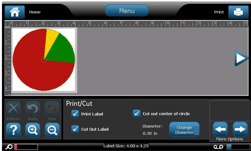
To help find the center of the gauge, in case the center of the gauge has a raised area, cut out the center of the circle of the gauge.
