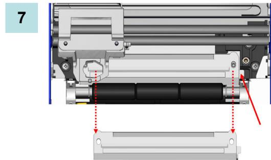
8. Use a moistened wipe from the cleaning kit to clean the cut pad.
