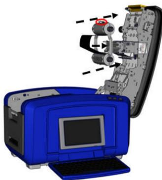
3. Turn the ribbon spindle knob to tighten the ribbon over the printhead.
