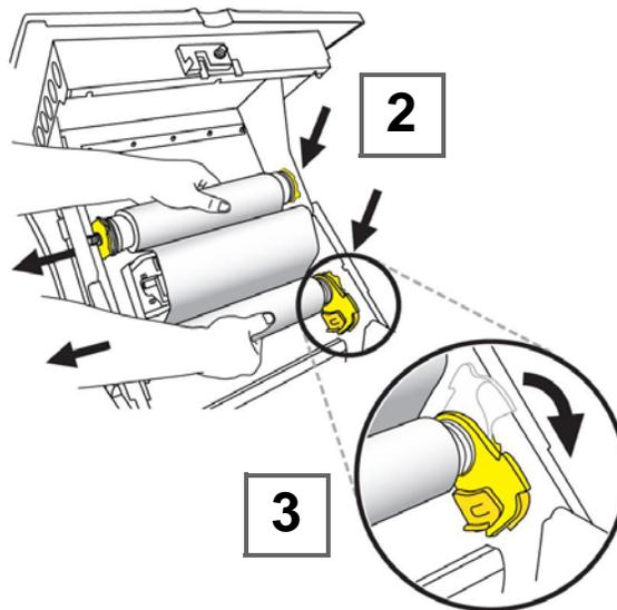
4. Place left side of media roll insert over yellow drive cone, pull toward left, then insert end of roll over opposite drive cone [4].
