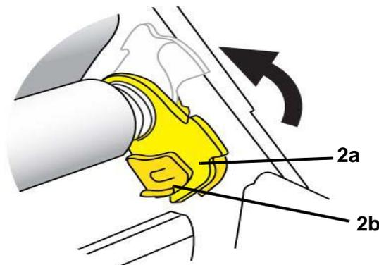
4. While compressing spring on left side of printer, grasp both sides of cartridge case and pull it toward you, then lift cartridge out of printer.
