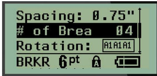
3. In the *Spacing*: field, enter the width of a standard breaker.
