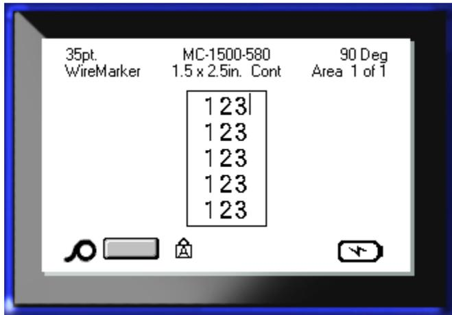
**Figure 33 • Repeated data on a WireMarker label**
