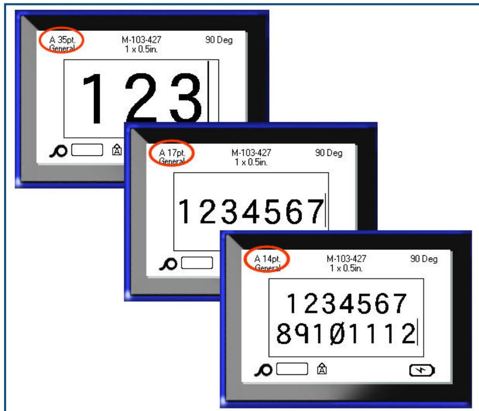
Figure 12 • Text entered with Autosize turned on
