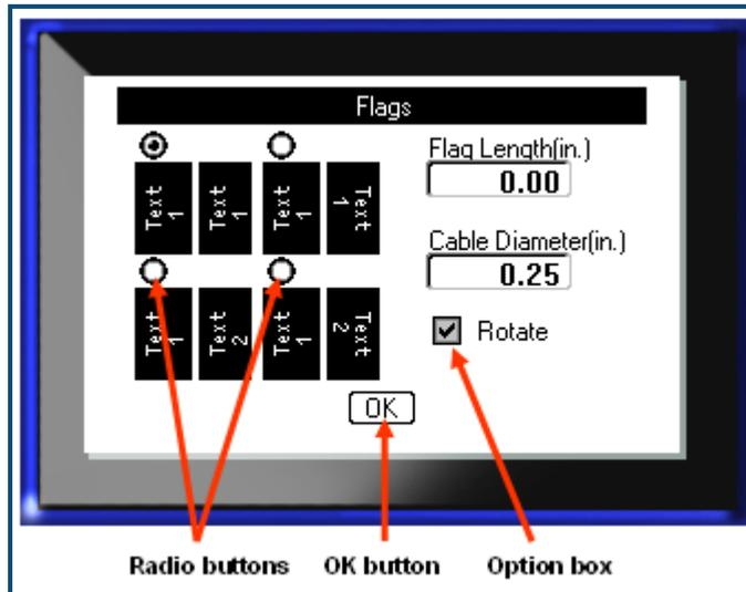
Figure 7 • Radio buttons, Option boxes and OK button
