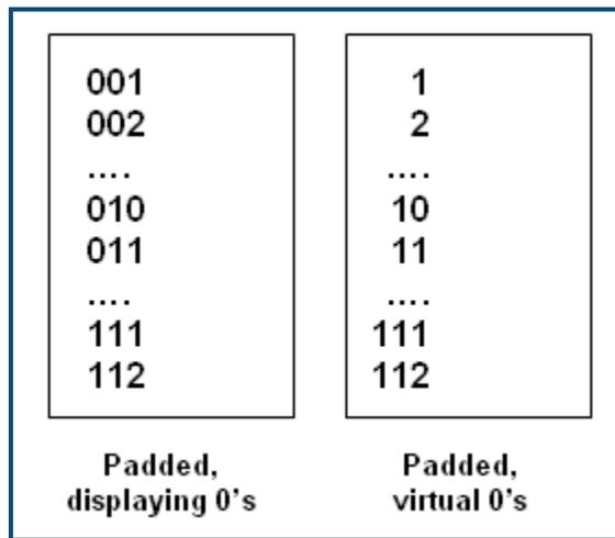
**Figure 26 • Displayed vs. virtual zeros in sequences**
