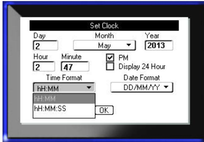
Figure 10 • Time/Date settings in Setup function
