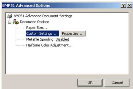
6. On the Custom Settings screen, click the down arrow in Cutter Option field and select if you want to pause the printer for cutting at the end of each label or at the end of the job.
