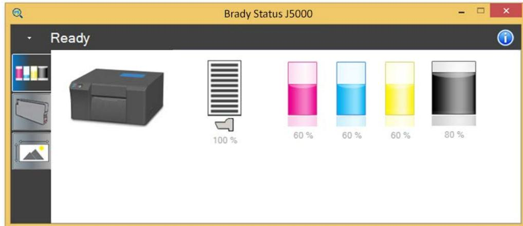
In the Ready mode, the ink percentages and printhead life will be displayed, along with three tabs. The tabs will only be displayed if the printer is Ready (not printing).
