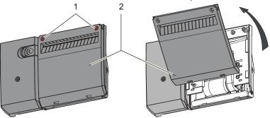
2. Loosen screws (1) and remove cover (2) towards the front.
