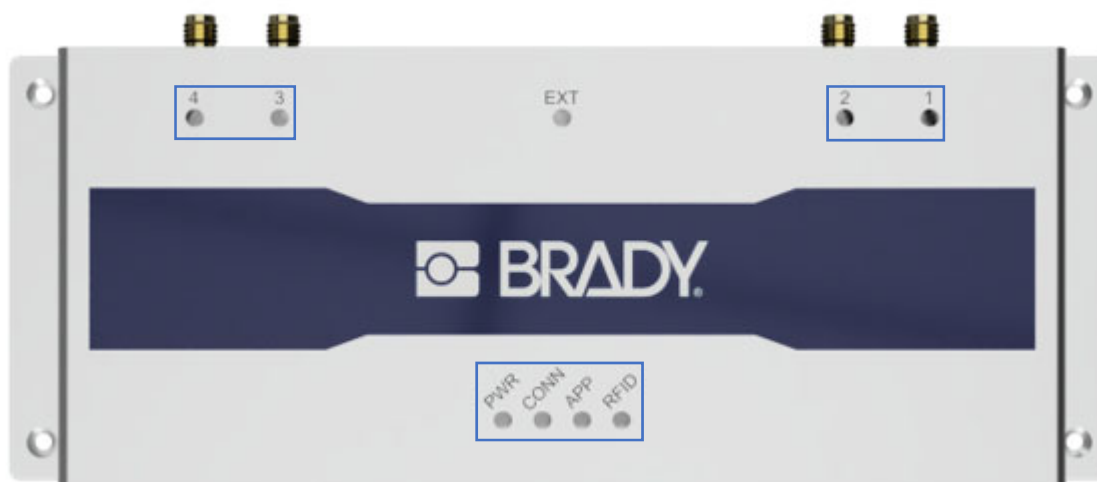
Picture 5 Location of LEDs
