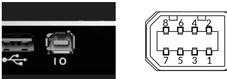
Picture 3 and Figure 1 Pin-out of the mini-IO connector on the Brady FR22 Lite rear panel
