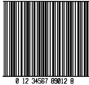
Bar Code L Interleaved 2 of 5 w/module 10 checksum and shipping bearer bars
