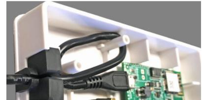
3. Insert the grommet around the cord, and slide into the grommet channel.
