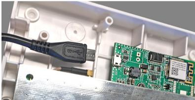
1. Insert the Micro-USB plus into the port on the reader board.
