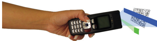
Too close to code.
