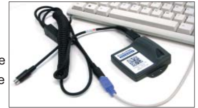
PS2 Cable installed to CodeXML Modem & Keyboard
