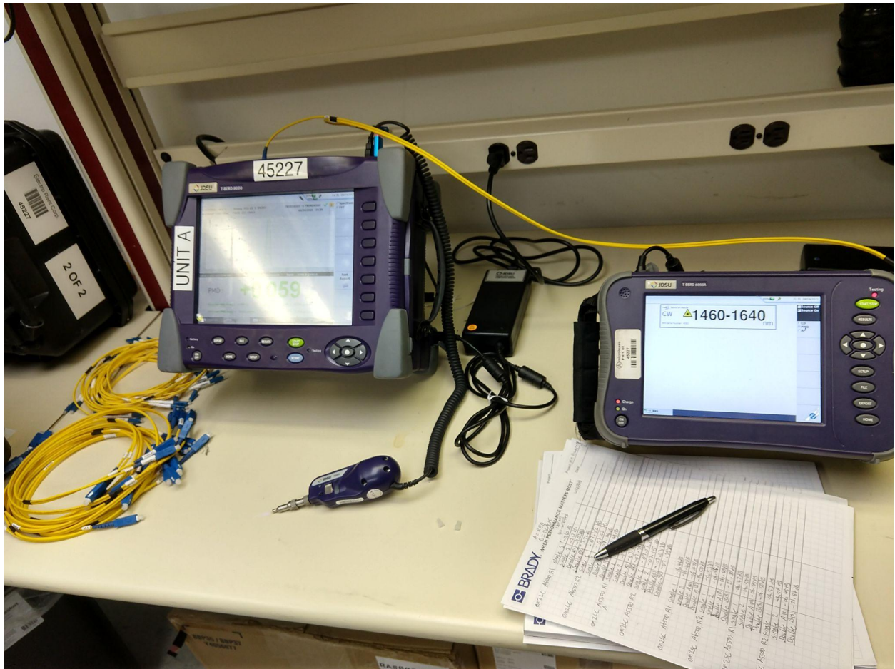
Figure 2. Tier 2 Test setup. Cable connects between T-BERD8000 (LEFT) and T-BERD6000A (RIGHT).
