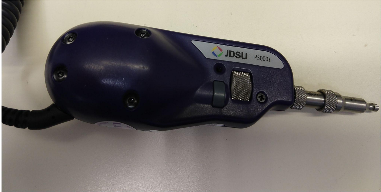
Figure 1. P5000i Fiber Microscope with SC connector attached
