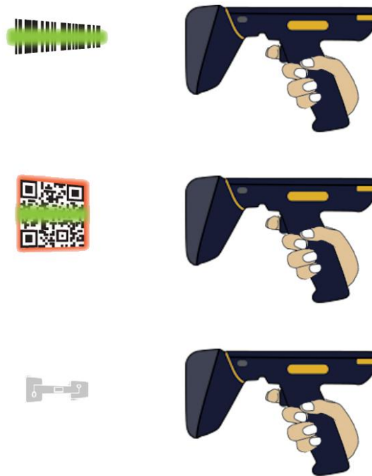
Figure 2-1. Handheld orientation for scanning barcodes and RFID tags
