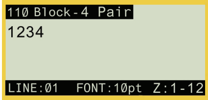
Display screen showing Zone 1 of a 4PR, 12-zone label
