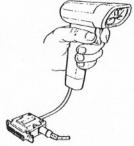
3. Turn the power ON on your labeling system and plug the bar code scanner power cord into an electrical outlet.
