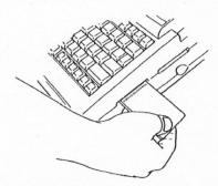
Follow this procedure to install a PowerCard. It is not necessary to turn the system off before inserting or removing a PowerCard. However, DO NOT insert or remove a card while the Card Active light is lit.
