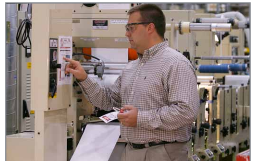
Having a written, visual lockout procedure at the point of need helps maintenance personnel quickly and accurately identify all control points.
