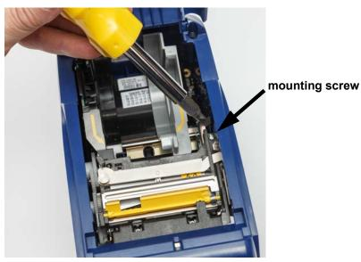
5. Loosen the mounting screw.
