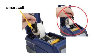
5. If using anything but a 2-inch (50 mm) wide label supply, slide the label guide to the left until it fits snugly up against the label roll and clicks into place.
