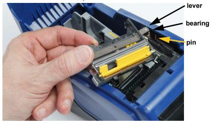
7. Install the new cutter assembly making sure the two tabs are located as indicated in the picture below, and the lever is between the bearing and pin on the actuator as shown in the picture above.
