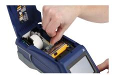
Make sure the print head is locked. Check the lock lever to make sure it is in position pointing toward the front of the printer.
