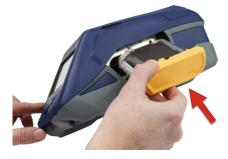
Turn the lock lever toward the front of the printer to lock it.
