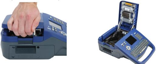
2. Remove the existing labels, if installed. Grasp the label roll and gently pull up out of the label well.
