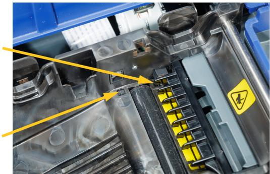
3. Using the pre-moistened cotton swab, gently wipe the sensors, located just before and below the ribs.
