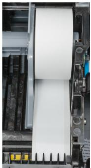
Figure 2-2. Position of leading edge of label supply.
