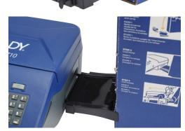
5. Open the printer and insert the label core making sure the smart cell on the label roll aligns with the reader in the label well.
