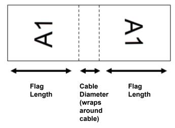
5. In the **Cable Diameter** field, enter the diameter of the wire or cable to which the flag will be applied.
