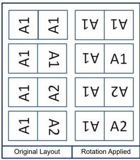
6. Rotate the data if desired. The provided layouts orient the text parallel to the wire or cable. If you want the text rotated 90°, select the **Rotate** check box.
