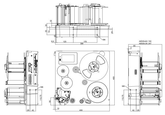
Figure 26 Assembly dimensions A8500
