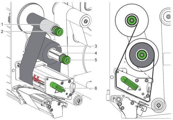
Figure 17 Loading transfer ribbon
