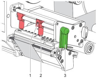
Figure 15 Setting the head locking system
