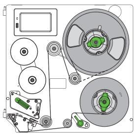
Figure 11 Inserting the labels into the print mechanism
