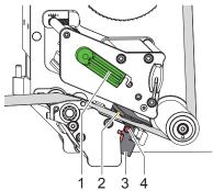
Figure 13 Setting the Label Sensor
