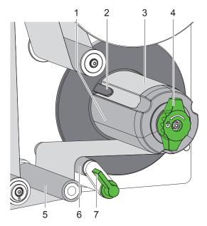
Figure 14 Guiding the liner to the internal rewinder
