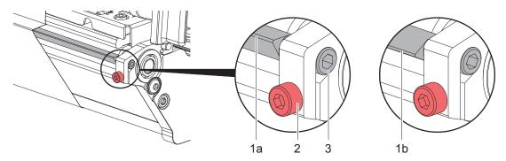
Figure 16 Setting the peel-off edge
