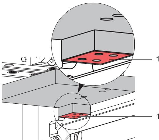
Fig. 5 Cleaning the pad with slide foil
