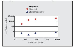
This data confirms that for standard labels the measured voltage on a label increases as the size of the label increases. For static dissipative labels, the voltage remains at a comparatively low level even as the label size increases.
