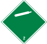
Non-flammable Non-poisonous Gas B-946 09025 Styrene 09045
