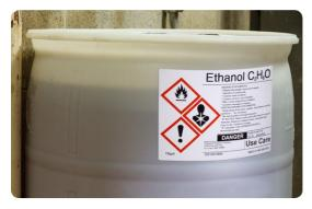
Carry out a review of all hazardous materials that are located around your worksite. Was it easy to identify potentially harmful materials? Hazardous chemical labels aid easy identification of substance classification. Current safety data sheets (SDS) for hazardous chemicals should also be available to communicate hazard information to employees, customers and emergency responders.
