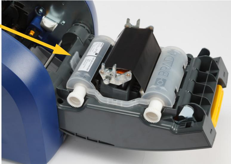
3. Place the ribbon cartridge so that the ribbon is over the printhead and the embossed Brady logo is facing upward. Snap the cartridge into place. You'll hear a click when it is seated properly.
