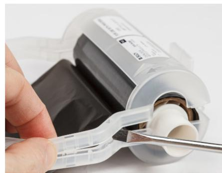
Repeat this process on both sides of the cartridge until all tabs are disconnected and the cartridge opens.
