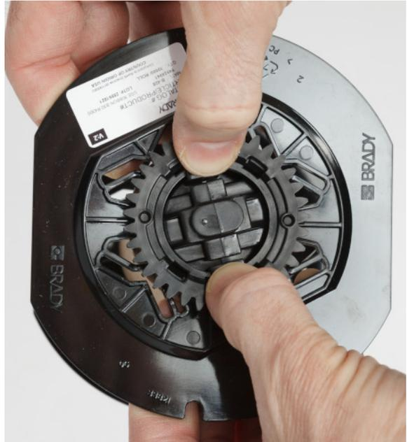
5. Push the screwdriver blade between the flat cartridge guides and **locking end cap**. Twist the screwdriver and continue this process around the end cap until it comes off.
