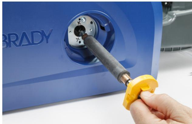
6. Insert the new print roller into the printer.
