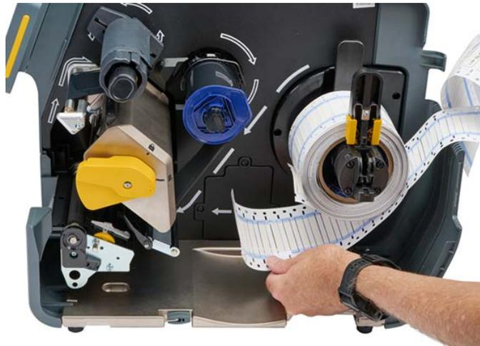
**Note:** Take care to insert the correct end of the strip for second-side print pass - “first sleeve first.”
