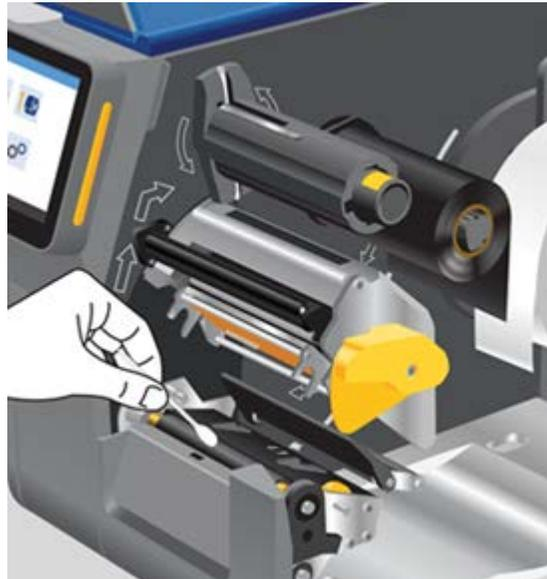
4. Replace the ribbon and label roll after the alcohol evaporates.
