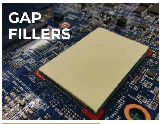
Soft Gap Filler is a soft material designed to conduct heat away from uneven surfaces. The conformability allows for intimate contact over rough surfaces and eliminates air.
